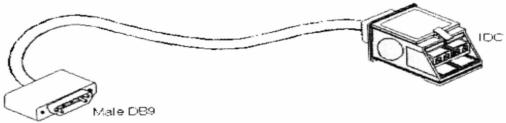
Type 1 IBM Cabling with IDC Connector for MAU and Male DB9 Connector for Peripheral Equipment
